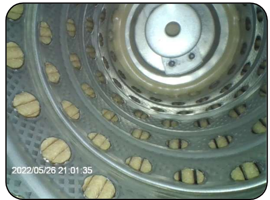
Oil Filter inspection using a Hawkeye Q Video Borescope
