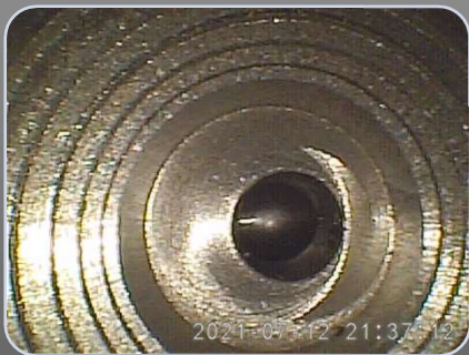
Thread and cross hole inspection in a machined part using a E-Series Video Borescope
