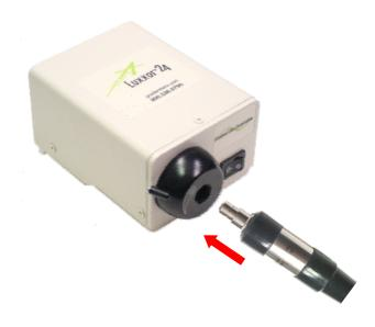
Connect the other end of the Luxxor® Light Guide to your Hawkeye® borescope by pushing it onto the light post of the scope until it clicks into place.
