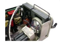
Pull the lamp back against the fingers, out of its cutout in the housing and slide it upward to remove it from the housing.
