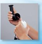
Clean the windows using a cotton swab dampened with Hawkeye lens cleaner, isopropyl alcohol or acetone.
