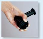
Push the borescope's eyecup into the housing and release the locking ring. Reverse to remove the borescope.
