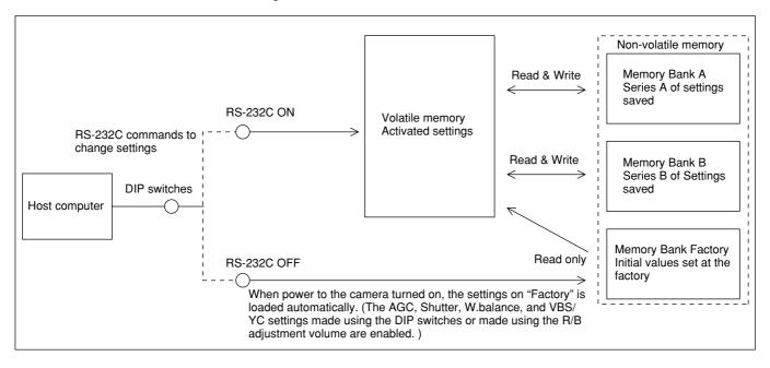
The XC-555 is equipped with three Memory Banks (Factory/A/B) to hold camera settings. Factory is "read only," holding the settings made when the camera was shipped from the factory. A and B can be written to, as well as read from, and the user utilizes these locations to hold setting values, calling them up when needed.
