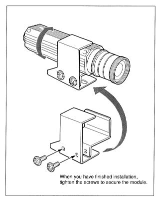
When mounting the camera on a tripod, use the supplied tripod adaptor.
