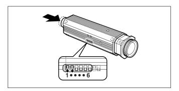
**5** Push the back panel and the CCD head block back into their previous positions, and tighten the Philips screws (7) to a torque of 0.18 N•m.
