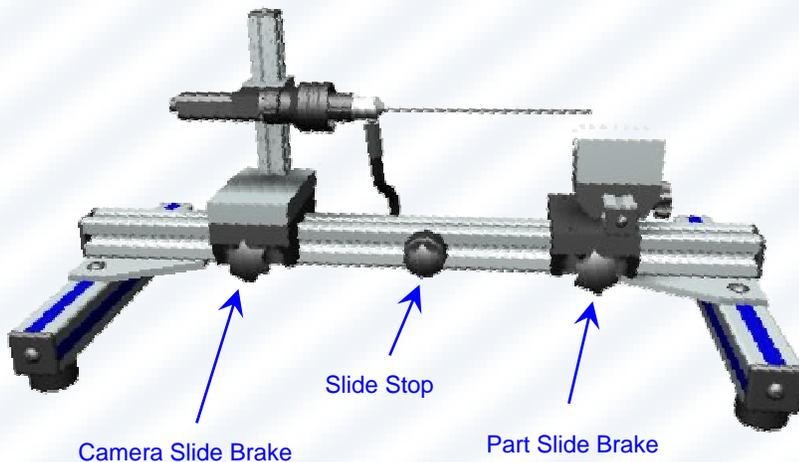
In either case, carefully position the slides so that the Borescope is at the maximum safe depth into the part. Tighten the brake on the slide chosen to be stationary. Then loosen the knob on the Slide Stop and move the stop until it is in contact with the slide chosen to be the moving slide. Tighten it down. Now as long as subsequent parts are mounted in the same position, the moving slide can be run until it contacts the stop without damaging the Borescope or the part.
