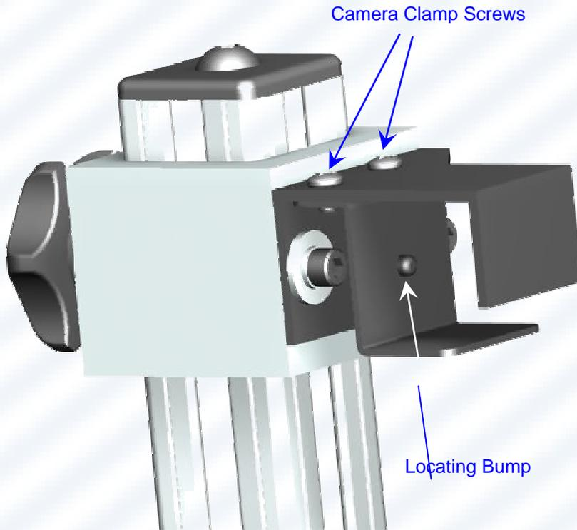
Loosen the Camera Clamp Screws 1 to 2 turns using a #2 Phillips screw driver. The screws are very short and will come out if turned too far. Be careful not to lose the screws.
