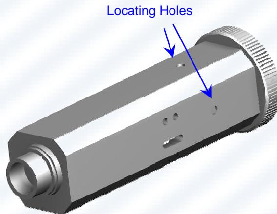
With the Camera Clamp Screws loosened, slide the Camera and Video Coupler into the Camera Clamp with the Camera Configuration Switches facing out as shown, so the image will be right side up.
