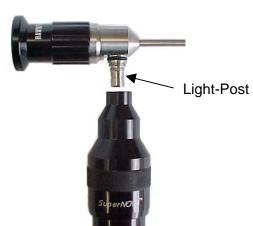
PUSH the SuperNOVA onto the light-post until the threads make contact, then turn. Screw the SuperNOVA onto the light-post until it is slightly snug against the borescope body.
