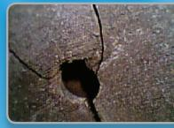
Using the Close-Focus tip, fine cracks are detected inside a combustion chamber.
