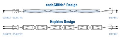
Our patented endoGRINs<sup>®</sup> gradient index lenses are the core technology of Hawkeye<sup>®</sup> Pro and Classic Rigid Borescopes. The elegant simplicity of the endoGRINs design gives excellent optical quality at a much lower cost than traditional alternatives, like the Hopkins design, which uses many expensive micro-lenses and optical glass rods.
