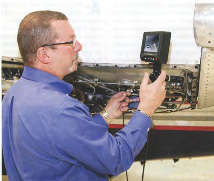
Cooling holes are examined during a combustion chamber inspection using a Hawkeye V2 Videoscope.
