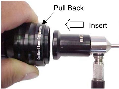
Focus the Hawkeye® borescope by rotating the eyecup.
