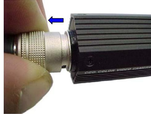
Once the cable is connected to the camera, locate the S-Video connector at the other end of the cable.
